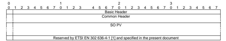
Figure 3: The SHB packet header format as specified in ETSI EN 302 636-4-1 [1]
